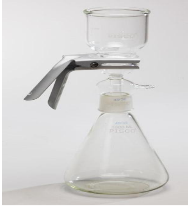
Figure 2. 1: Membrane filtration unit.
