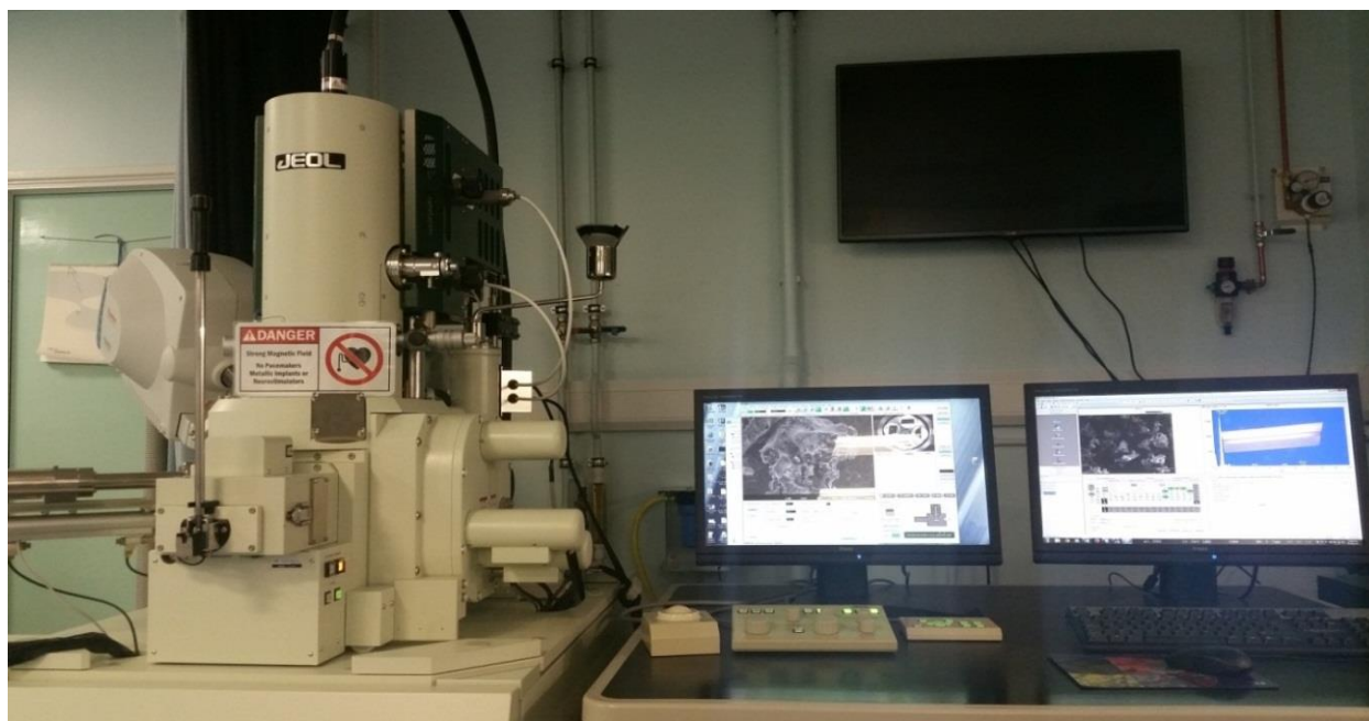
Figure 3.2: A photograph of a scanning electron microscope (JEOL, JMS 7100F) used in this study (Courtesy of the Department of Mechanical Engineering, University of Surrey, UK)
