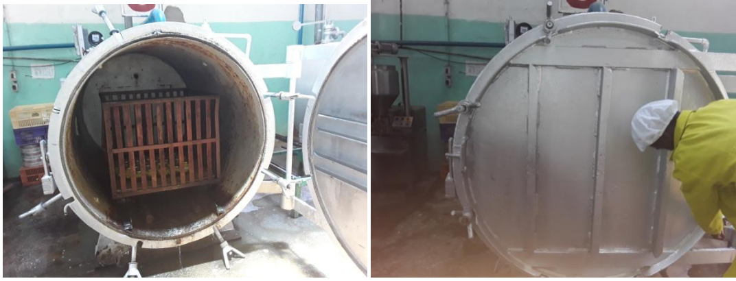
Plate 1. 5 Sterilization of the chunks in a retort
