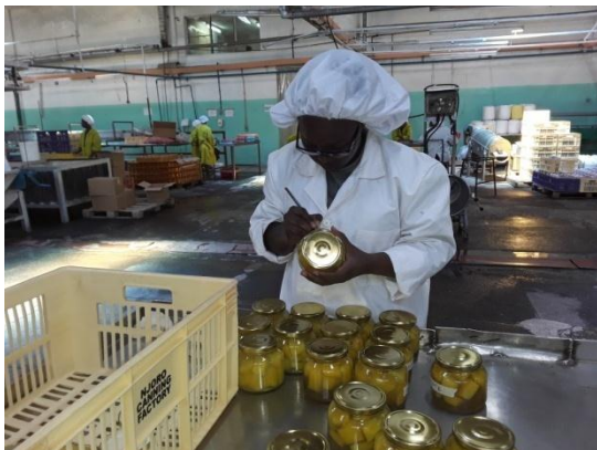
Plate 1. 4 Sealing and labeling glass jars
