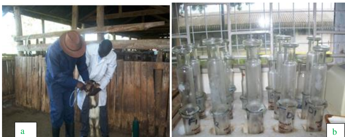
Figure 4. Process of rumen liquor extraction and in vitro incubation in 100ml calibrated glass syringes
