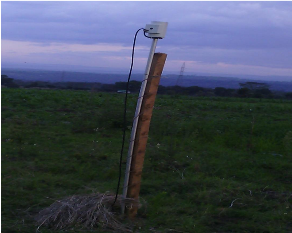
Figure 4.1: G-856 magnetometer set to take readings at the base station
