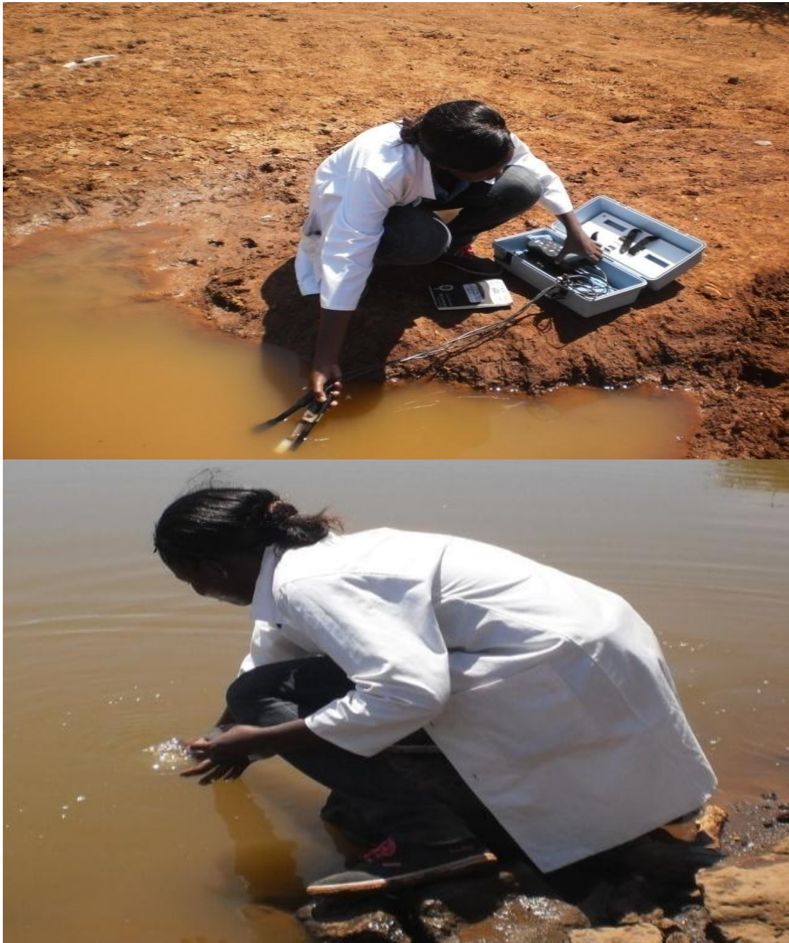
Plate 3.1: Plates of sampling showing: (a) The student researcher reading the physical-chemical parameters using WTWO microprocessor PH/temperature and conductivity meter: (b) The student researcher sampling water at Chepnyorgin water pan
