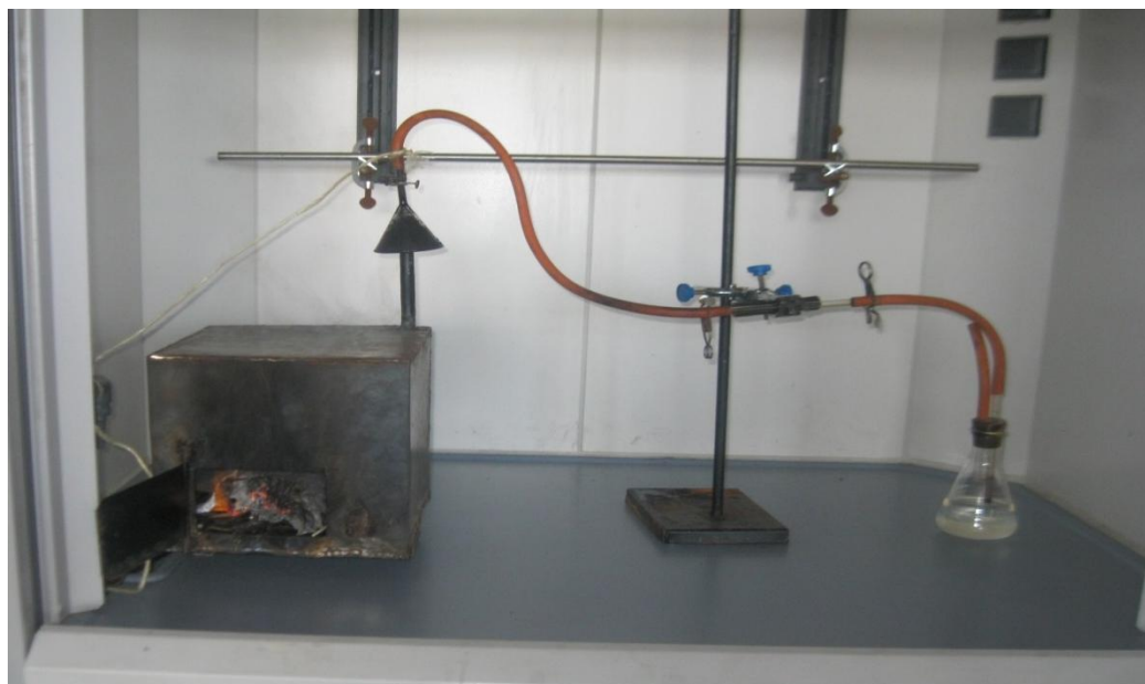
Figure 3.1: Reactor assembly for the simulation of a forest fire
