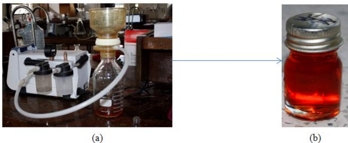
Figure 6. (a) Vacuum pump extraction of formazan from soil sample, (b) an extract of formazan from soil sample ready for spectrophotometric analysis.
