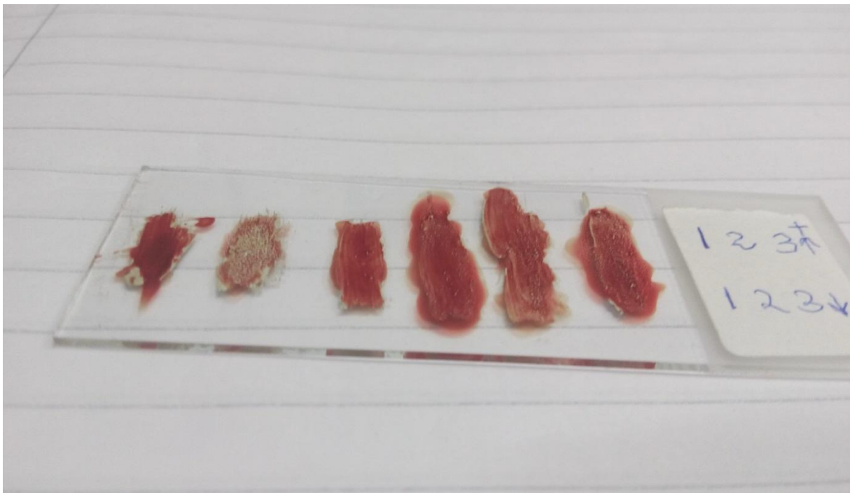
Plate 4: Blood samples adsorbed on Ag substrate on a microscope glass slide
