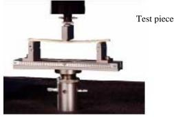
**Figure 1: Three-point bend test set up** Egerton J. Sci. & Technol. Volume 12: 146-154
