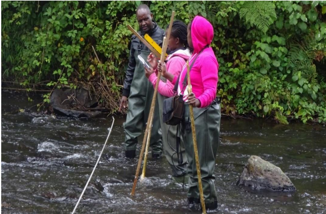
Plate 4- 11: Measurement of discharge in the Kamweti River.
