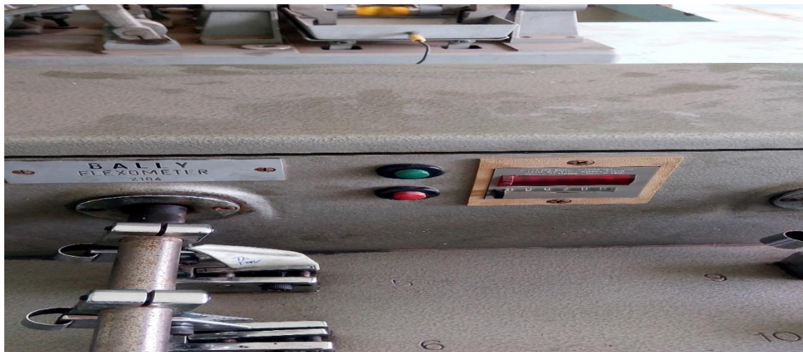
Plate 3.6: The actual sample folded and fixed in a flexometer
