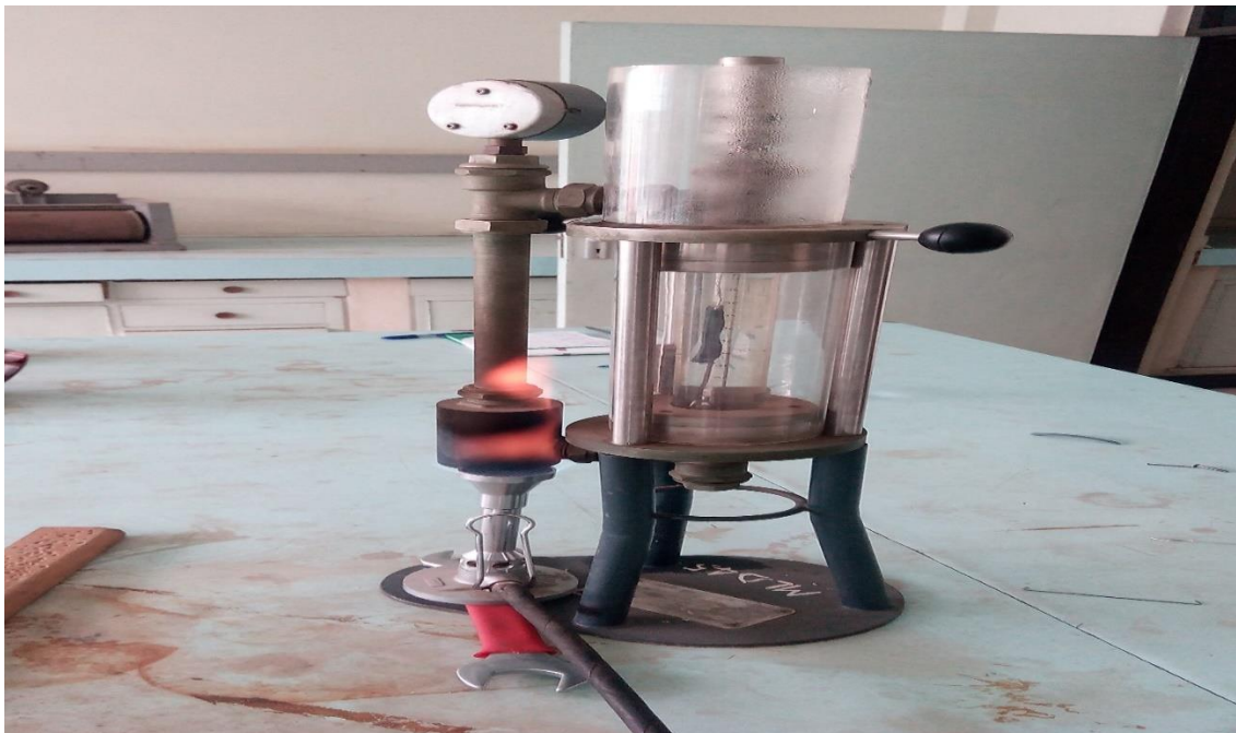
Plate 3.7: The arrangement of shrinkage temperature apparatus
