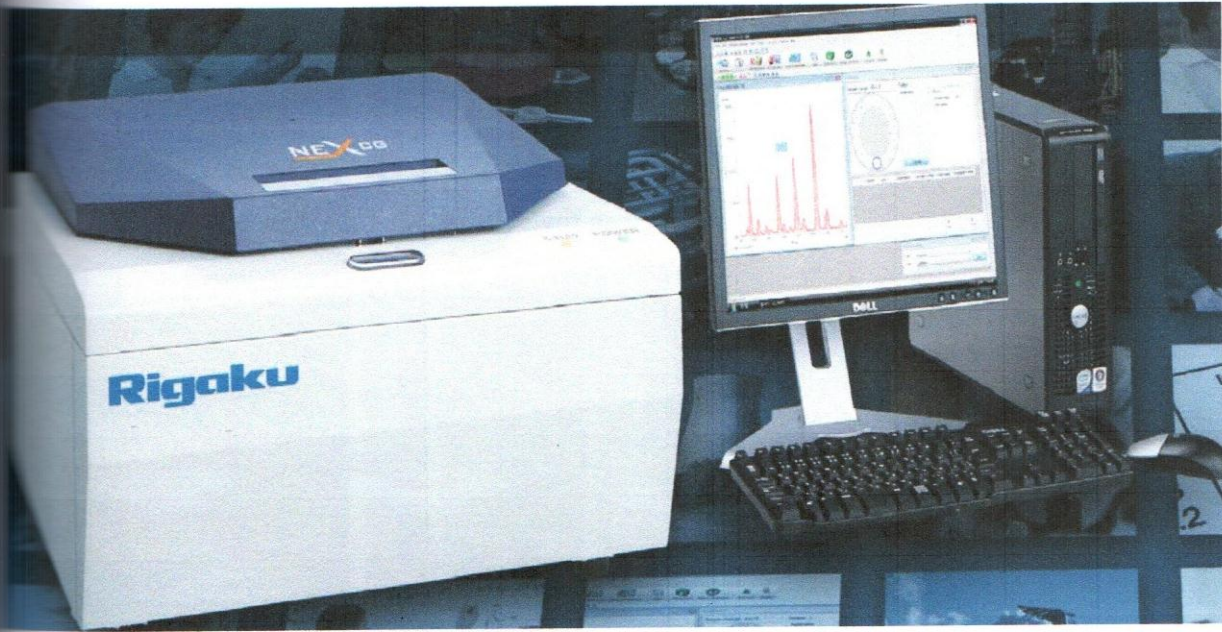
Plate 3.10: The Rigaku NEX CG spectrometer and PC system
