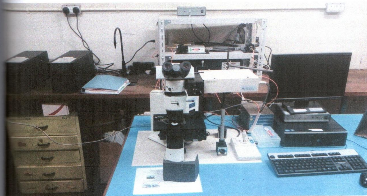
Plate 3.8: Confocal Raman Microscope with spectrometer
